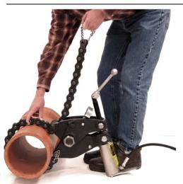
Using hand ring, pull chain over pipe and under tie bolt, then up between jaws as tightly as possible. Allow chain to relax so nearest pin is engaged in slots under upper nose jaw. Chain then can be folded over on itself.
