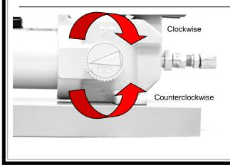
9. Turn valve clockwise on the pump until it is HAND TIGHT. DO NOT USE A WRENCH. Make strokes necessary to snap pipe. Turn knob counterclockwise to release valve after cut to retract piston.
