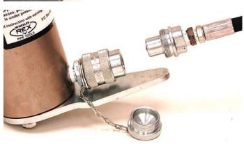
8. Attach hydraulic pump to cylinder. Remove dust cover from coupling, insert hydraulic hose end and turn threaded coupling sleeve until tight by hand.
