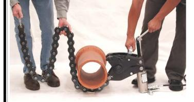
2. Slide chain under pipe at location of cut.
