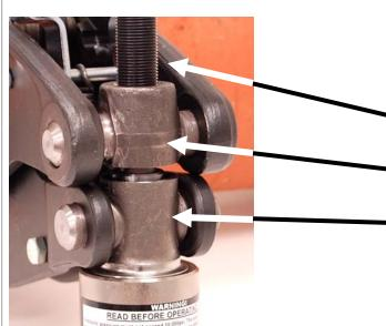
Turn adjusting screw until outer collar is at it's lowest limit of travel. Do this for EACH cut.
