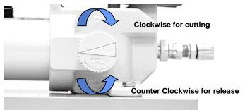
8. Turn valve clockwise on the pump until it is HAND TIGHT. DO NOT USE A WRENCH. Make strokes necessary to snap pipe. Release valve after cut to retract piston.
